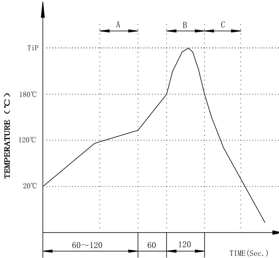
A.Preheating B.Soldering C.Gradual Cooling
