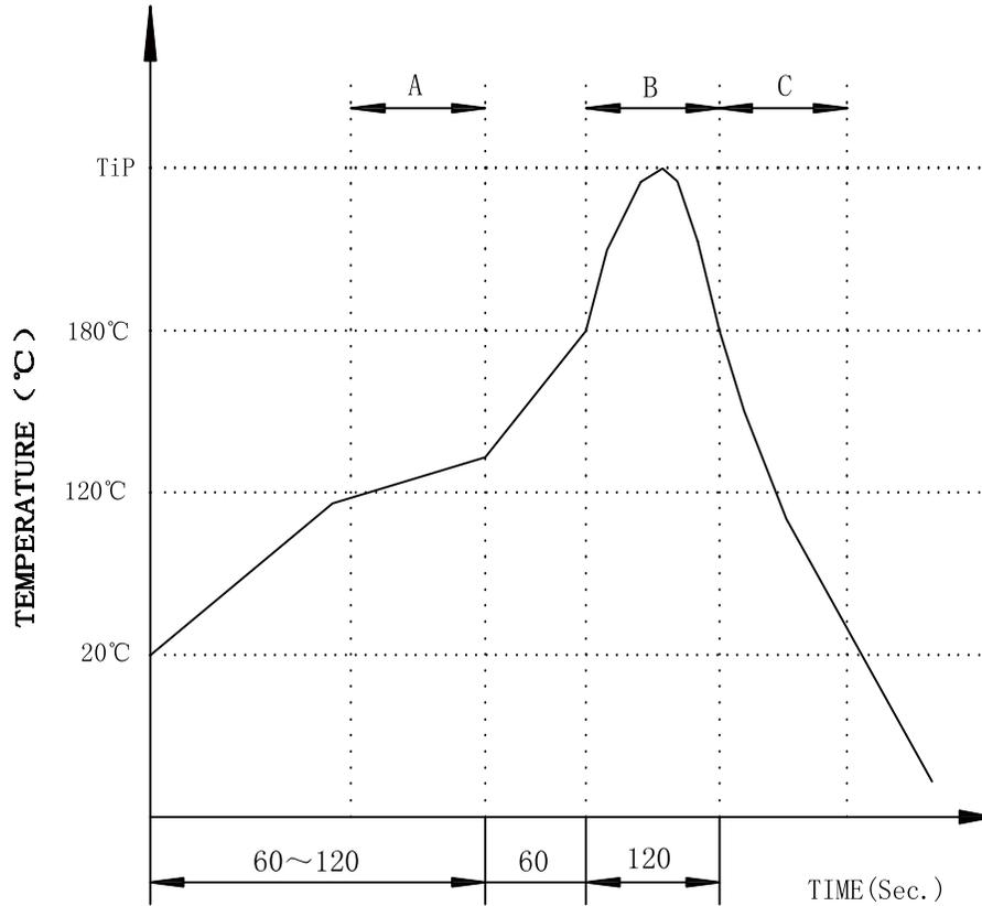
A.Preheating B.Soldering C.Gradual Cooling
